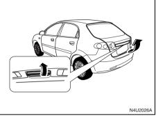
To open the liftgate, pull up the handle above the license plate.
